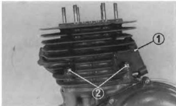
Fig. 3-11 (1) Cylinder (2) Nuts (four)
