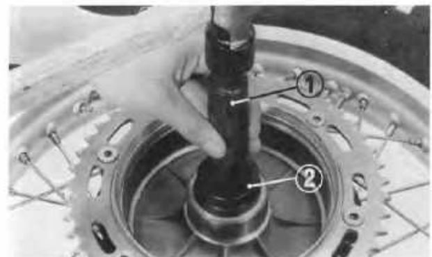
Fig. 4-39 (1) Driver handle (2) Bearing driver attachment
