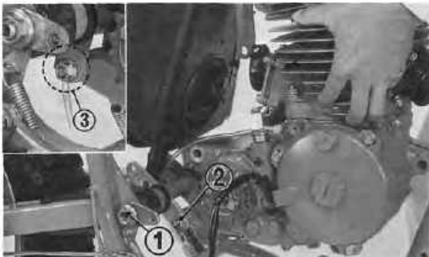
Fig. 3-7 (1) Swingarm pivot bolt (2) Engine mounting (3) Nut
