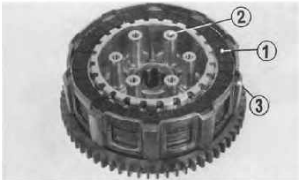
Fig. 3-28 (1) Clutch disc (2) Clutch center (3) Clutch outer
