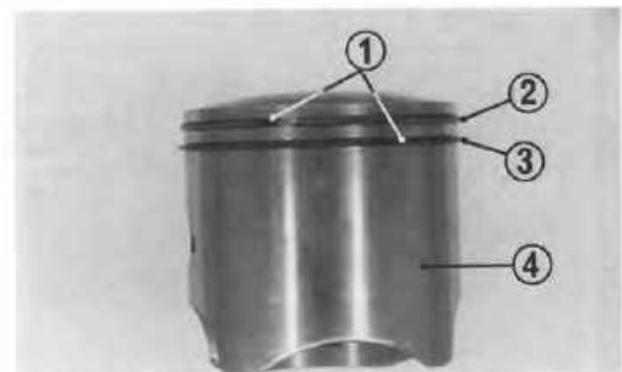
Fig. 3-20 (1) Piston ring stopper (2) Top ring (3) Second ring (4) Piston
