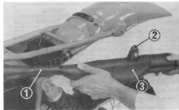
Fig. 6-3 (1) Rubber protector (2) Muffler hanger (3) Spark arrester
