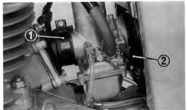
Fig. 3-2 (1) Carburetor insulator band (2) Air intake tube band
