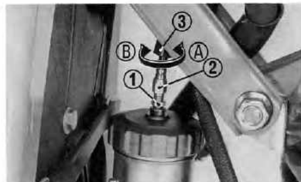
Fig. 2-19 (1) Lock nut (2) Adjuster (3) Rubber cap
