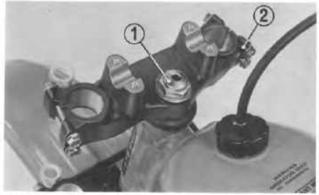
Fig. 4-3 (1) Steering stem nut (2) Fork top bridge
