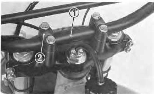
Fig. 2-25 (1) Handlebar (2) Handle upper holder
